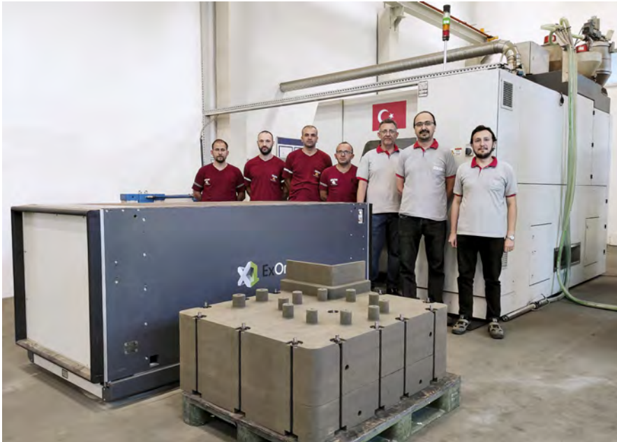
Döktas 3D Printer engineering and operation team. The S-Max Pro is the fastest and high-volume 3D sand printer of its kind.
